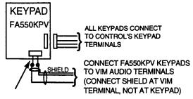
USE SA550AB AUDIO CONNECTOR SPLICED TO SHIELDED CABLE WHEN USING FA550KPV KEYPAD
